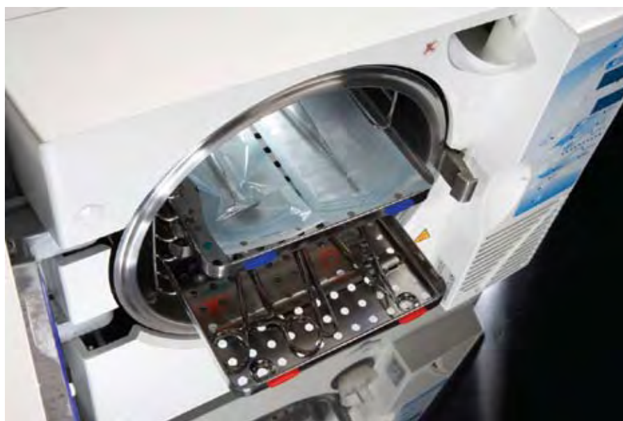
● A new generation vacuum autoclave showing how pouched instruments are accommodated.
