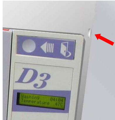
Fig 1. Location of access plug covering door release hole
